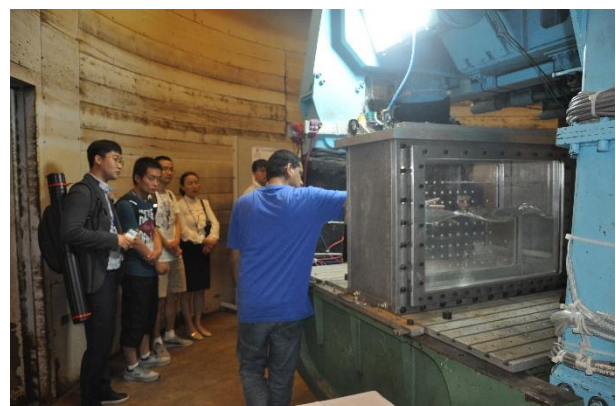
Figure 9. Students showcasing a new wave tank equipped in the HKUST geotechnical centrifuge for offshore foundation testing
