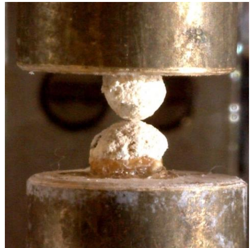
Two weathered volcanic grains under uniaxial compression
