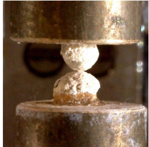
Two weathered volcanic grains under uniaxial compression
