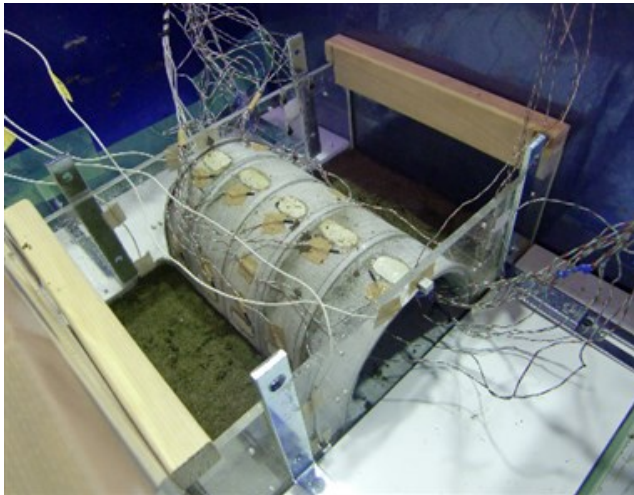
Figure 4. Centrifuge model test (arch culvert)
