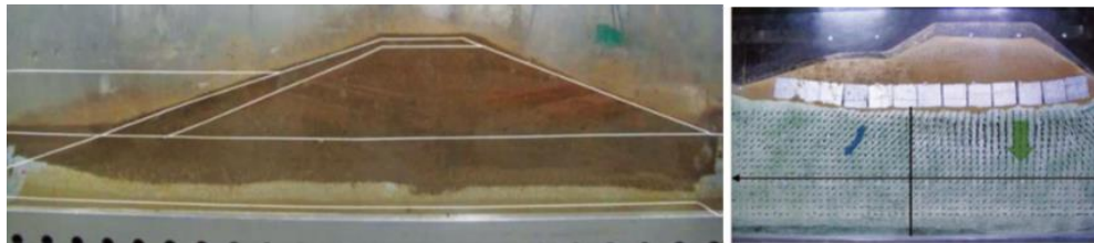
Figure 13. Embankment seepage & settlement analysis.
