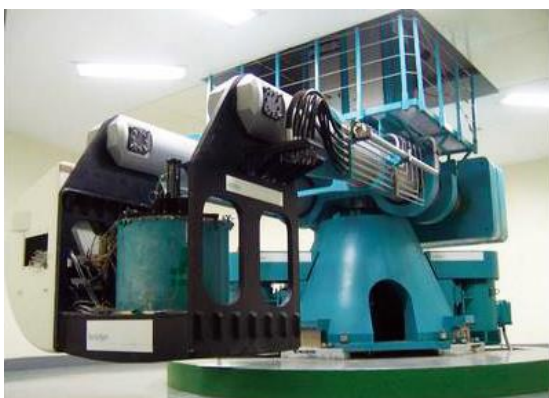
Figure 7. KOCEDs geotechnical centrifuge
