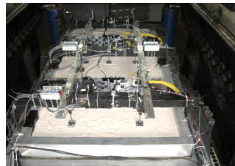
Models of retaining walls for testing
