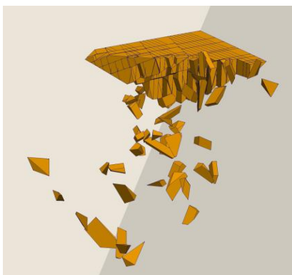
DEM model of disintegration of a jointed rock mass
