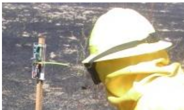
Early mote prototype for wildfire monitoring
