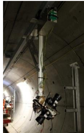
Computer vision for tunnel inspection
