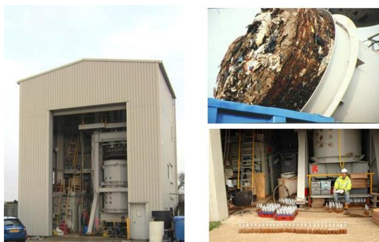
Figure 6. Southampton's 2m-diameter waste compression cell.
